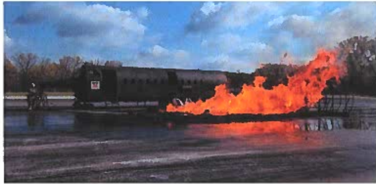
Fuel spill pan fires
