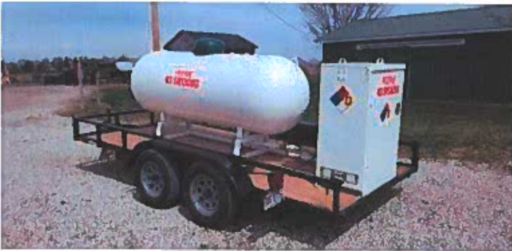
LPG fueling system to fuel props (mobile version shown)
